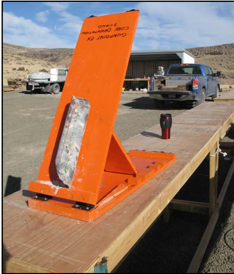
Figure 10.6 Core Orientation Stand
