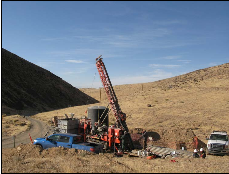
Figure 10.2 Diamond Drill Rig on the Talapoosa Project
